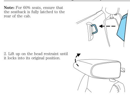
**WARNING:** Before returning the seatback to its original position, make sure that cargo or any objects are not trapped behind the seatback. After returning the seatback to its original position, pull on the seatback to ensure that it has fully latched. An unlatched seat may become dangerous in the event of a sudden stop or collision.
